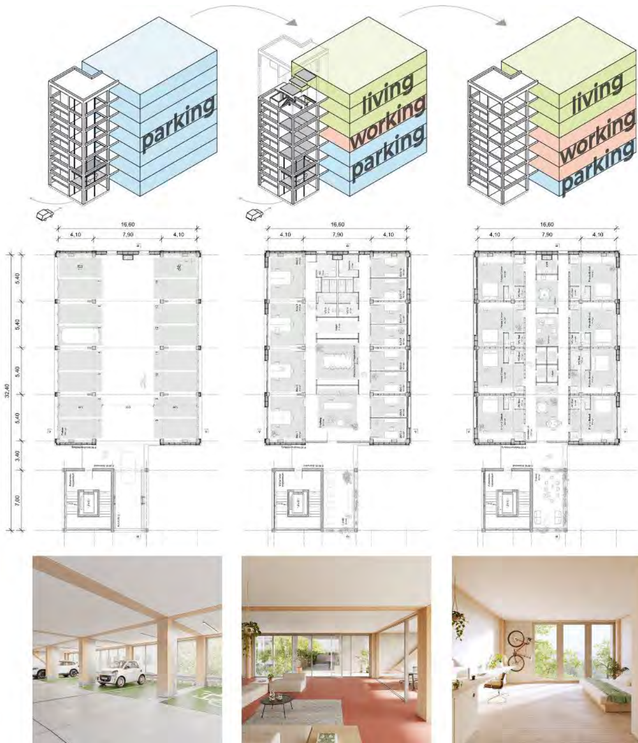
Image 7: Flexibility of use and implementation of parking, working and living spaces in the same structural framework. © t-lab, RPTU, Kaiserslautern-Landau / Nicolai Becker images
