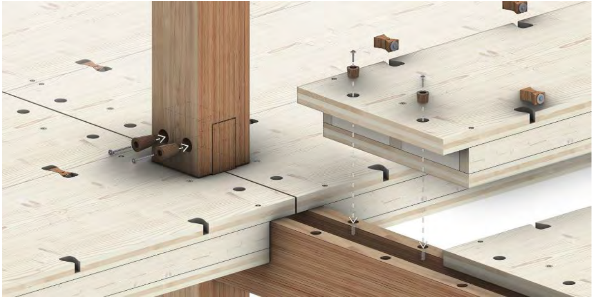
Image 8: Column, Beams, hollow core floor elements – Reversible Conical Adapters and P2P Connections. © t-lab, RPTU, Kaiserslautern-Landau
