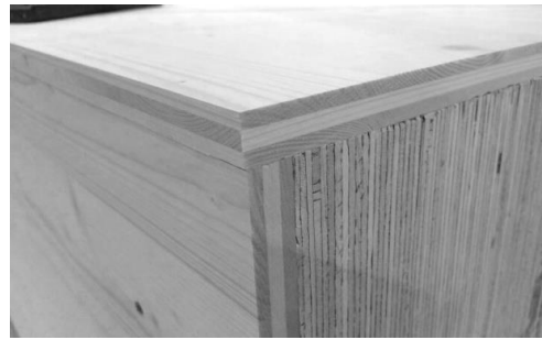
Figure 11: Prototype of re-glued LVL SOURCE: Stora Enso | R&D Building Solutions
