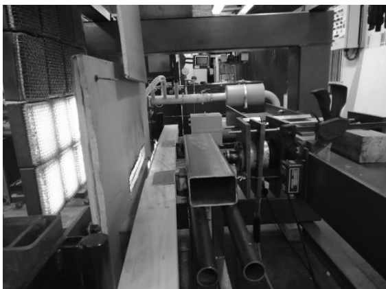
Figure 6: Fire test setup and loading apparatus.
