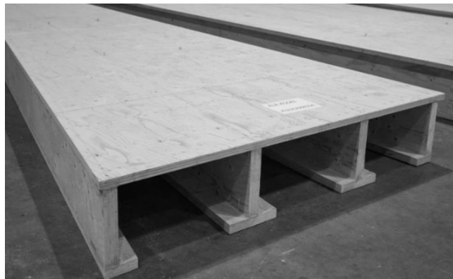
Figure 7: LVL Rib panel for Wood City in the prefabrication at Timberpoint Oy. SOURCE: Stora Enso; Timberpoint Oy
