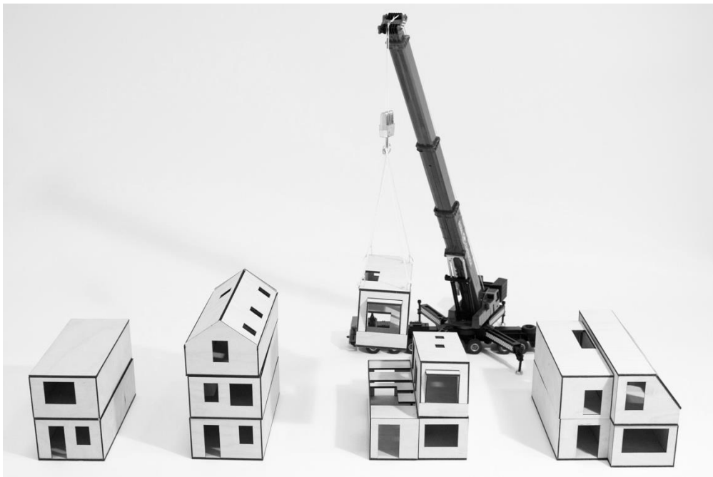
Image 7: prefabricated CLT modules
