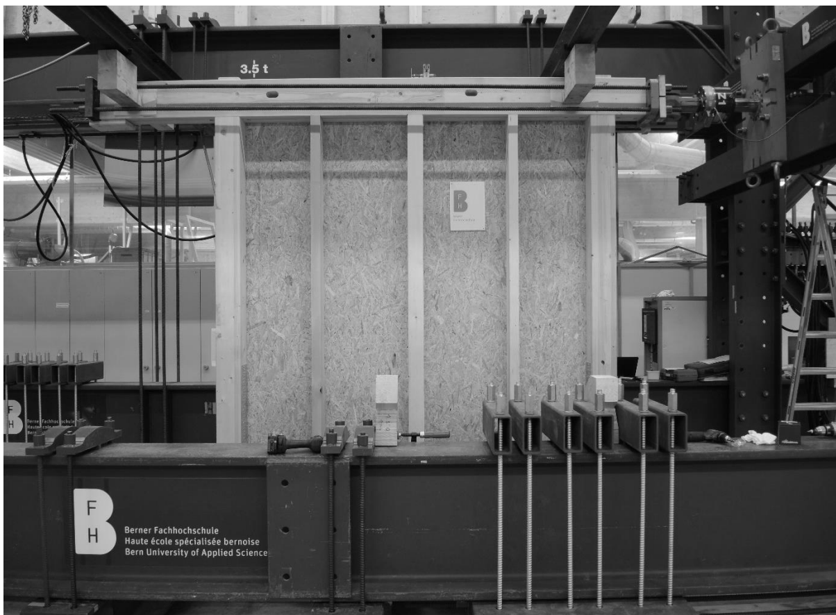
Figure 2: Timber frame shear wall "C2" during test in the laboratory at BUAS.
