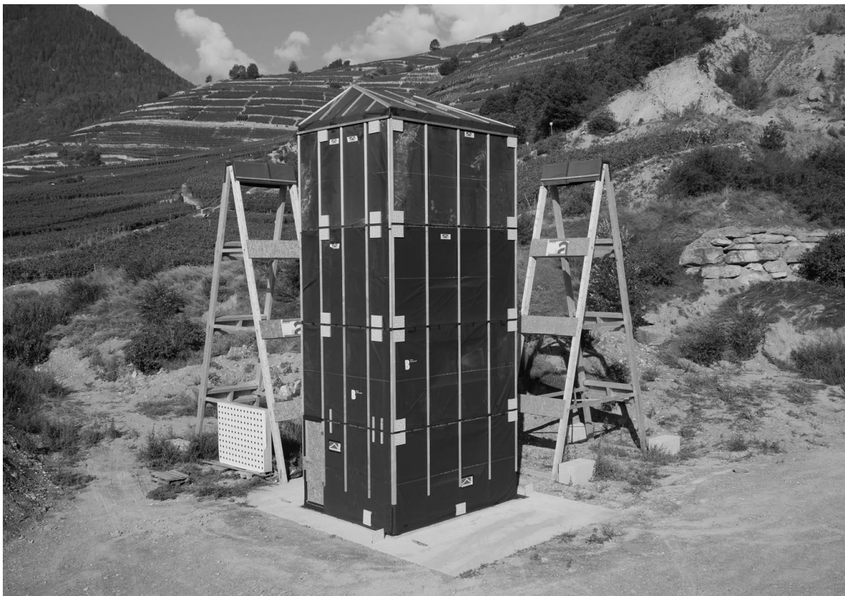
Figure 1: Experimental plant with 4 story building and racks for cable tensioning system.
