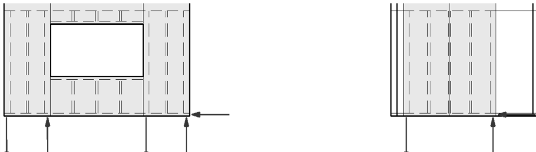
Figure 5: Action and reaction forces for two wall setups. On the left side: X-wall, right side: Y-wall.
