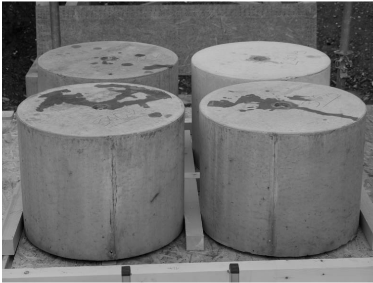
Figure 10: Prefabricated concrete blocks to simulate dead-load in a building.
