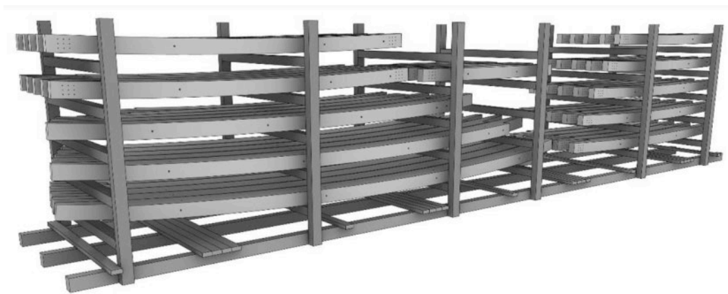
Figure 13: Individual Container of doubly curved Glulams, result of packing algorithm
