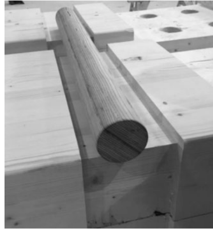
Figure 9: LVL beech dowel and timber cut-outs
