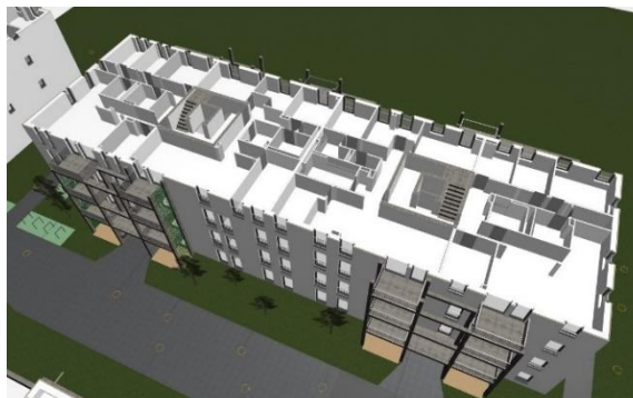
Abbildung 8: BIM Modell Zentrale Kerne WAS
