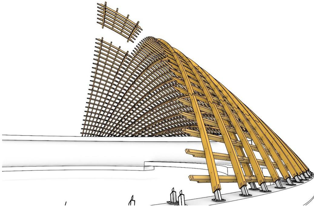
Figure 12: Pre-fabricated panel on the Large Dome
