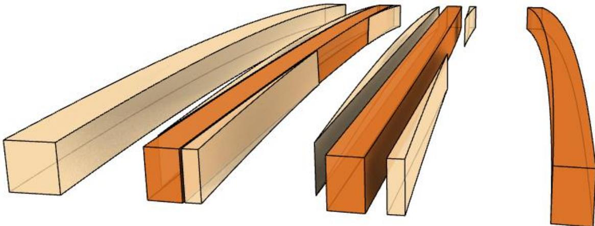
Figure 4: Doubly-curved Glulam elements made from singly-curved billets
