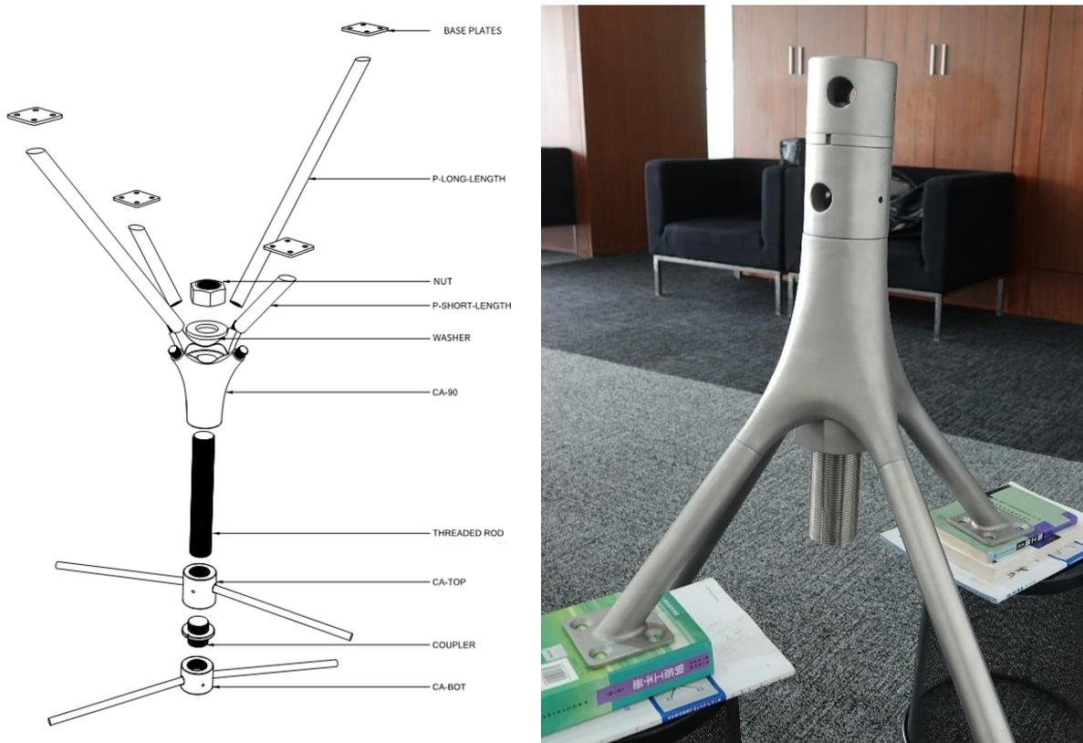
Figure 9: Arrangement of the King Post and Cable Assembly
