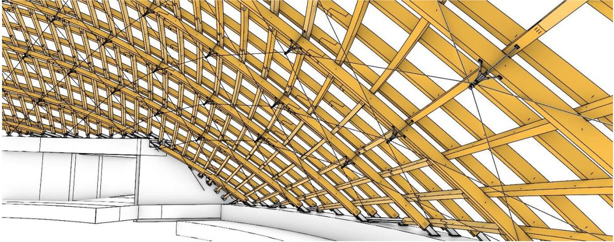
Figure 7: King post and cable arrangement in large dome
