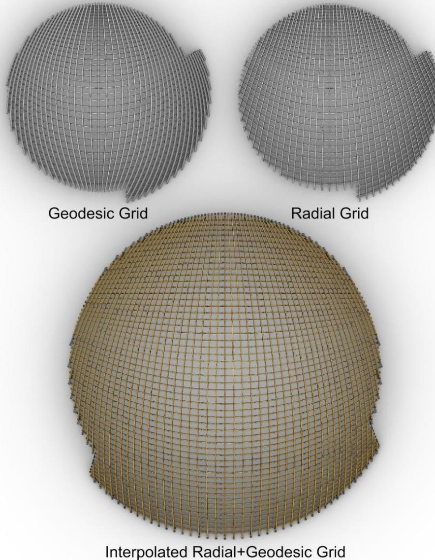
Figure 2: Geodesic Grid vs. Radial Grid for primary elements. Actual grid used was an interpolation between.
