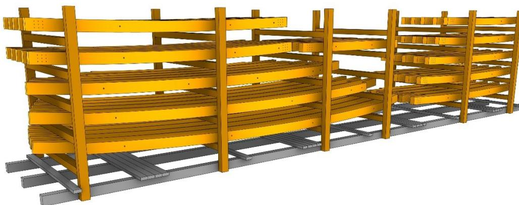
Figure 13: Individual Container of doubly curved Glulams, result of packing algorithm
