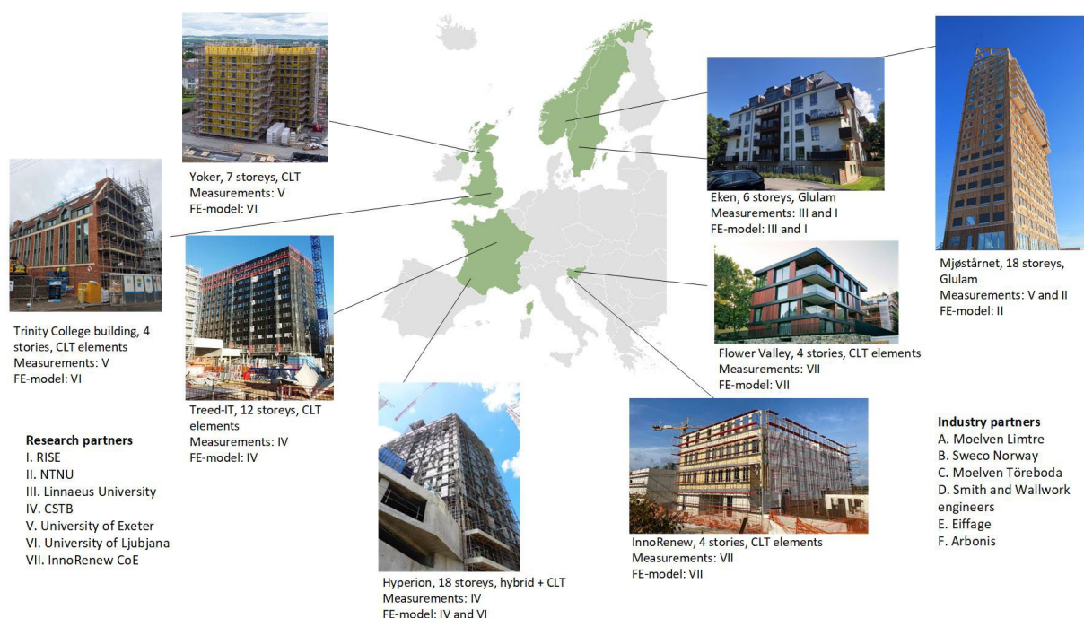
Figure 1: The buildings tested and their locations in Europe. Partner responsible for measurements and FE-modelling can also be seen below each building.
