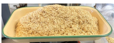
Figure 7: A fossil-free and full size IsoTimber panel was grinded to fibers and saw dust, that was used to produce OSB- and particleboards respectively in lab scale (0.2 x 0.2 m).
