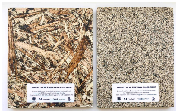
Figure 7: A fossil-free and full size IsoTimber panel was grinded to fibers and saw dust, that was used to produce OSB- and particleboards respectively in lab scale (0.2 x 0.2 m).
