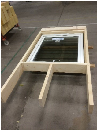
Figure 4: Prefabricated window module.
