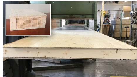
Figure 5: Full size (1.2 m x 2.4 m) fossil-free IsoTimber panel produced in industrial scale out of plywood in pilot scale (1.2 m x 1.2 m).
