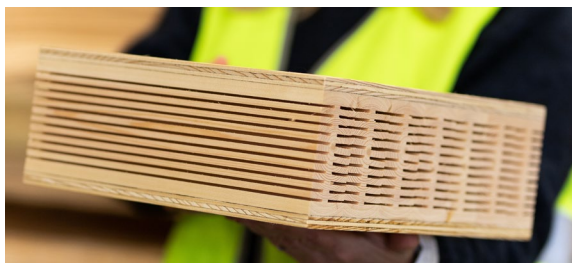
Figure 4: Small size (0.3 m x 0.3 m) fossil-free IsoTimber panel produced in lab scale.
