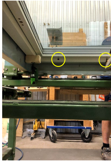
Figure 11: Closed window with anchor holes marked yellow.
