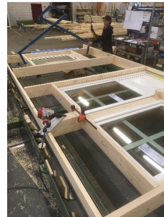
Figure 6: Assembly of window module into wall frame.
