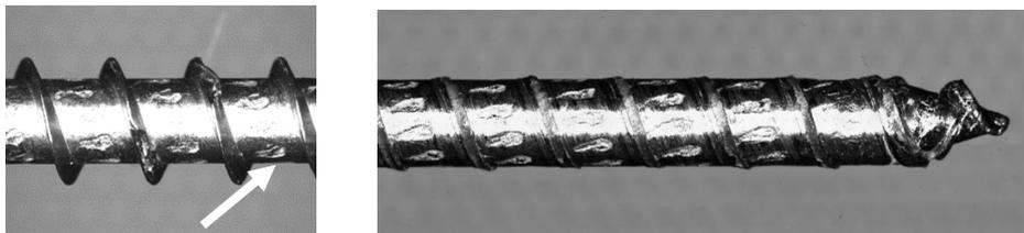
Figure 9: Damages to wood screws caused by mutual contact. Local damage to a firstly screwed-in screw (left) hit by a secondly screwed-in one (right) resulting in almost complete loss of the thread.
