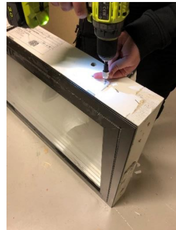
Figure 15: Attaching a plastic Click-In clip at a window frame.
