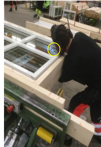
Figure 12: Closed window with operator in unergonomic position when drilling the screw (yellow-marked).
