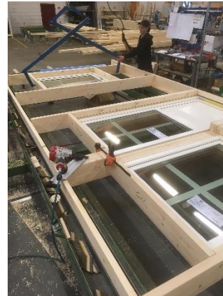
Figure 6: Assembly of window module into wall frame.
