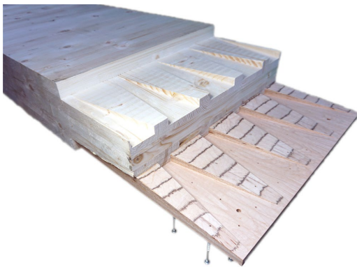
Figure 12: Milled CLT adherend with one-sided bonded beech LVL gusset plate with tapered fingers (alternative B)
