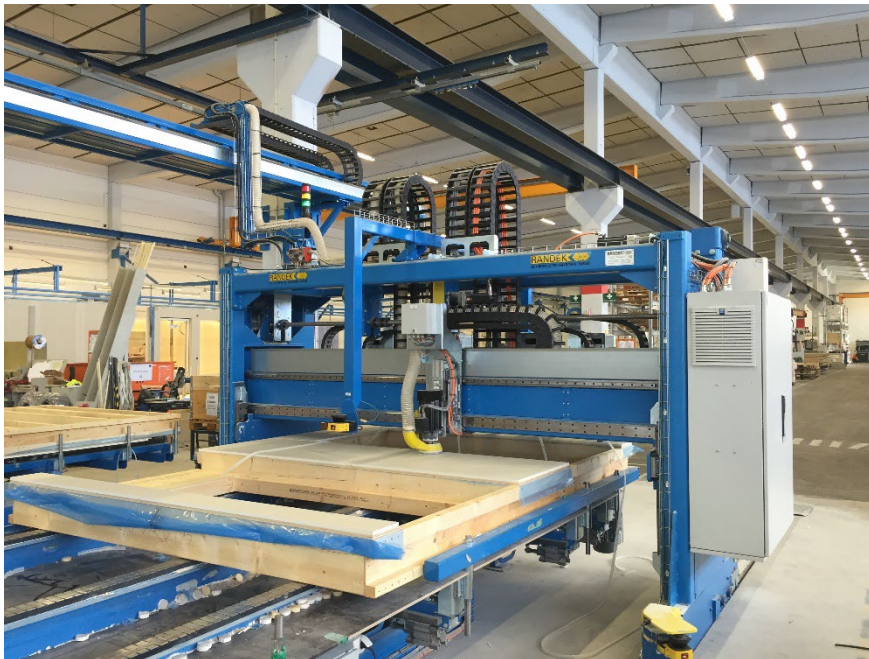
Figure 3: Automated machine producing wall elements in BoKlok's factory
