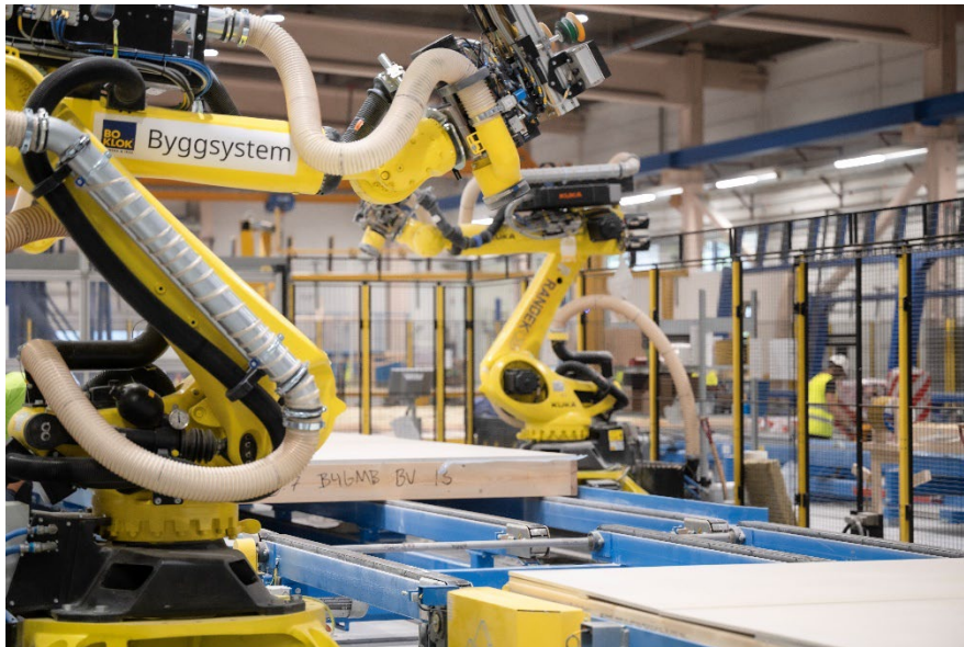
Figure 4: Robots working on wall panels
