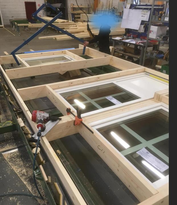
Placement of window modules in manual framingstation
