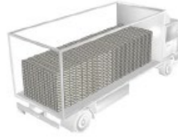
Figure 5: Transport of multiple prefabricated tooth beam lamellas
