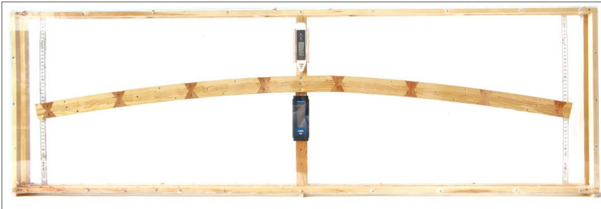
Figure 18: «HygroSim» testing set-up, a plexiglas box to observe beams under humid conditions
