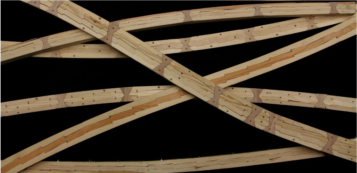
Figure 15: First physical tests for evaluation and approximation of a predefined target curvature
