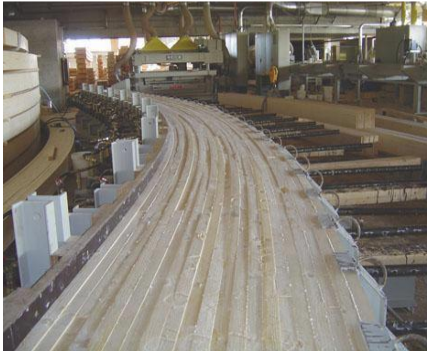
11 Curved glulam production, pressing
