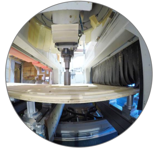
Milling tool: Diameter 10 cm
