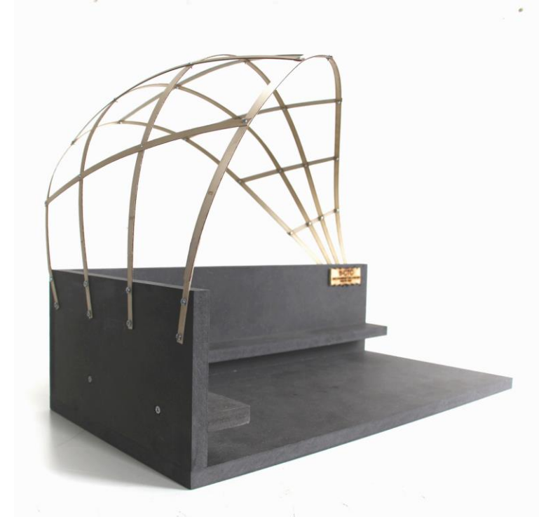
Increasing additional torsion, physical confirmation model
