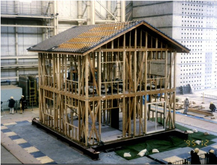
conventional framework construction
