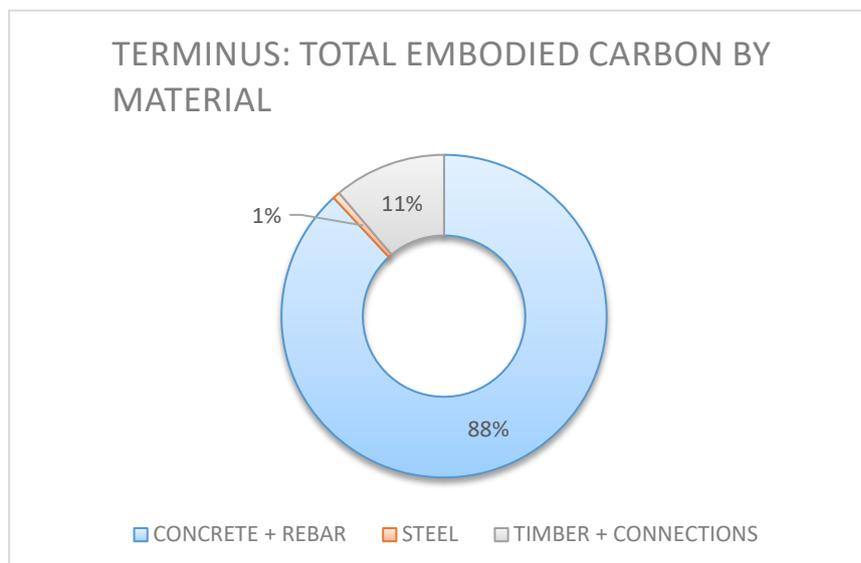
Figure 2: Terminus: Total Embodied Carbon by Material
