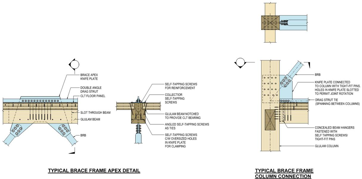
Figure 4: Terminus Brace Frame Connection Details
