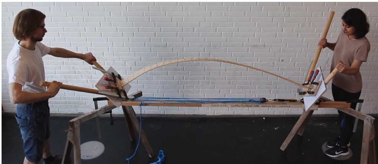
Figure 19: «BendMax-TwistoMat» testing set-up, to simultaneously bend and twist tooth beam lamellas
