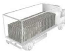
Figure 5: Transport of multiple prefabricated tooth beam lamellas
