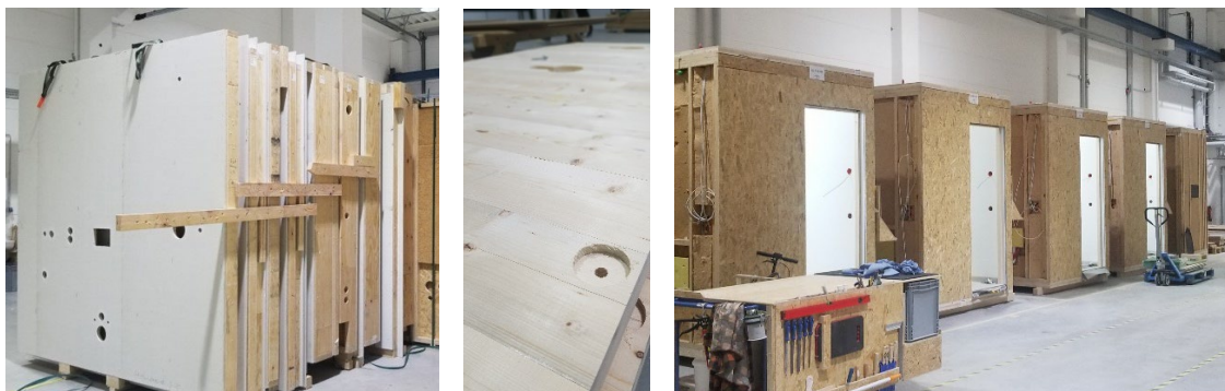
Figure 4.4.2: Prefab walls, CLT panels, and assembled modules from the POC. (Pictures courtesy of Tjiko)
