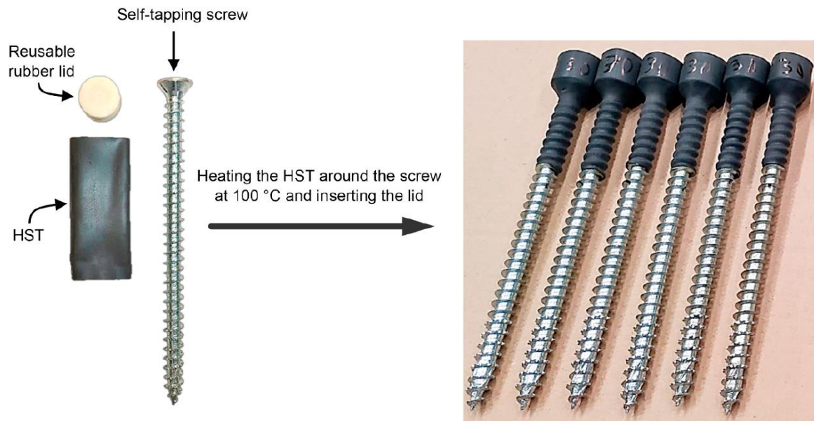
Figure 1: Deconstructable connector using self-tapping screws: individual components, production process, and final configurations [17].
