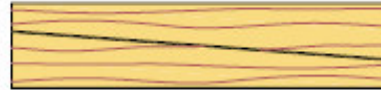
Figure 1.47. Principle of diagonal sawing of LVL panel to produce single-tapered column and gitter members of portal frames.
