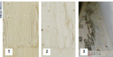
Figure 1.46. Appearance of LVL veneer surface. 1. Unsanded face side. 2. Optical sanded face side. 3. Calibration sanding revealing the dark glue line.
