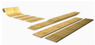
Figure 1.21. Composition of LVL, from veneer mat to cut-to-size panel.
