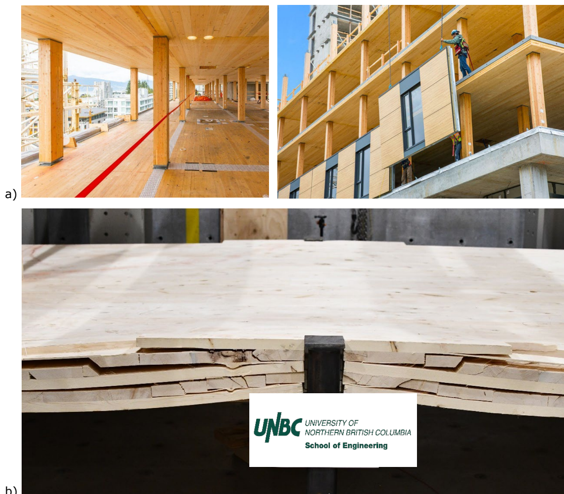
Figure 1: Point-supported CLT floor: a) UBC Tall-Wood house, © Fast+Epp; b) Punching shear failure
