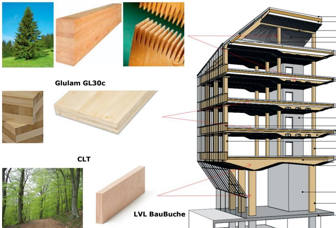
Figure 6: Different types of structural timber
