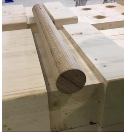
Figure 9: LVL beech dowel and timber cut-outs
