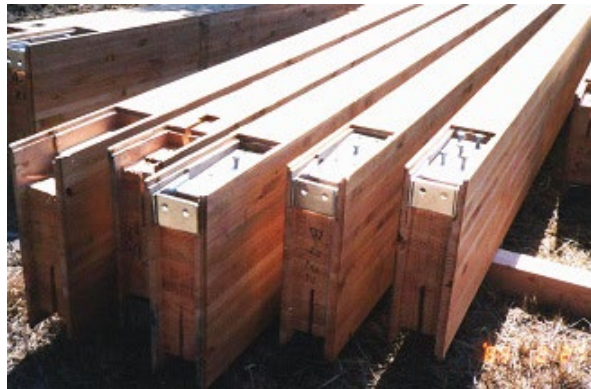
Prototype connection by BRI
