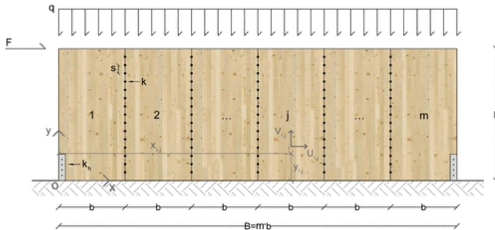
Figure 1: CLT Shear wall System<sup>1</sup>
