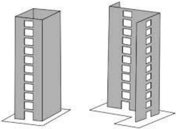
Figure 3: Concrete Shear Wall Configurations<sup>2</sup>
