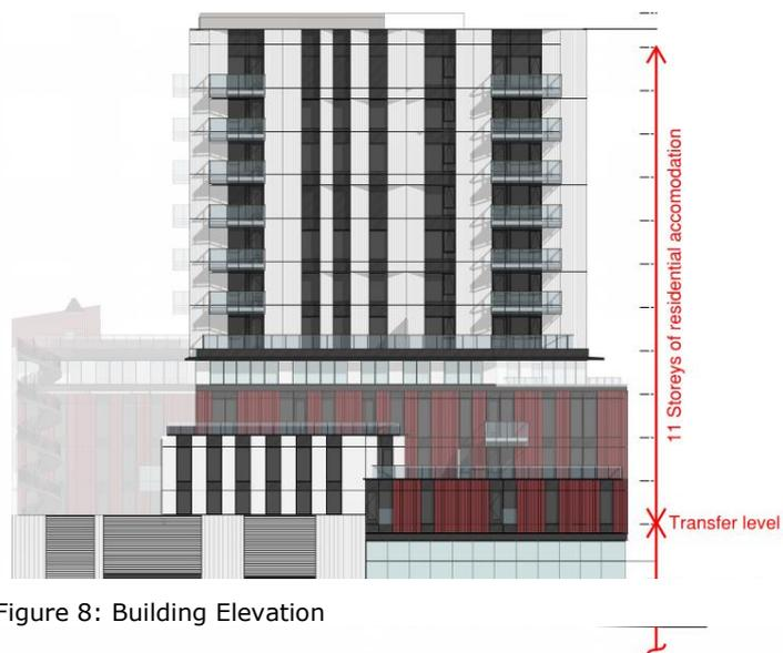
Figure 8: Building Elevation
