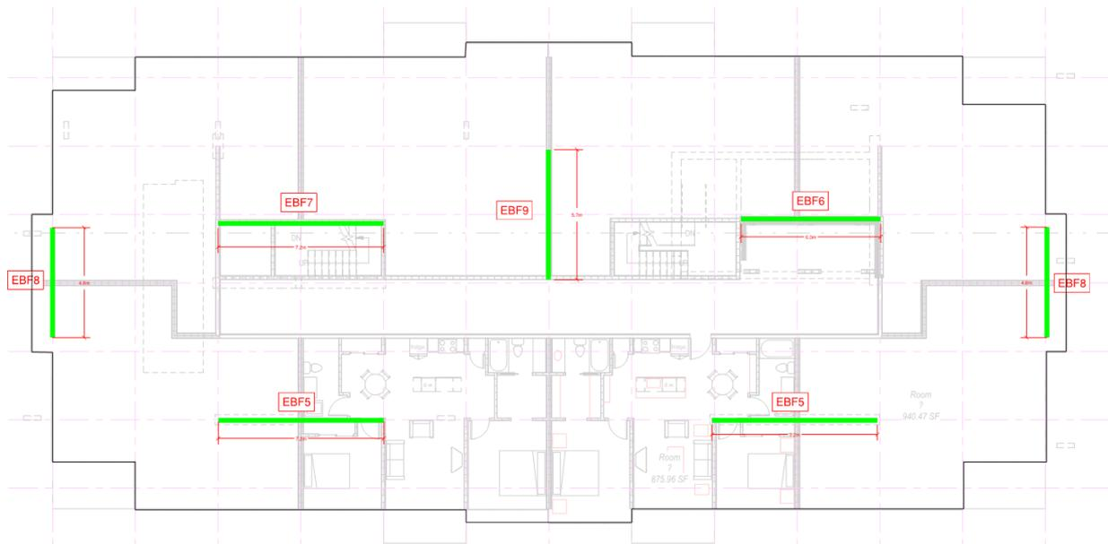
Figure 13: Floor Plan with Brace Locations
