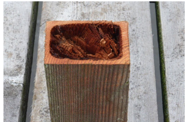
Figure 8: Fence Post Decay
